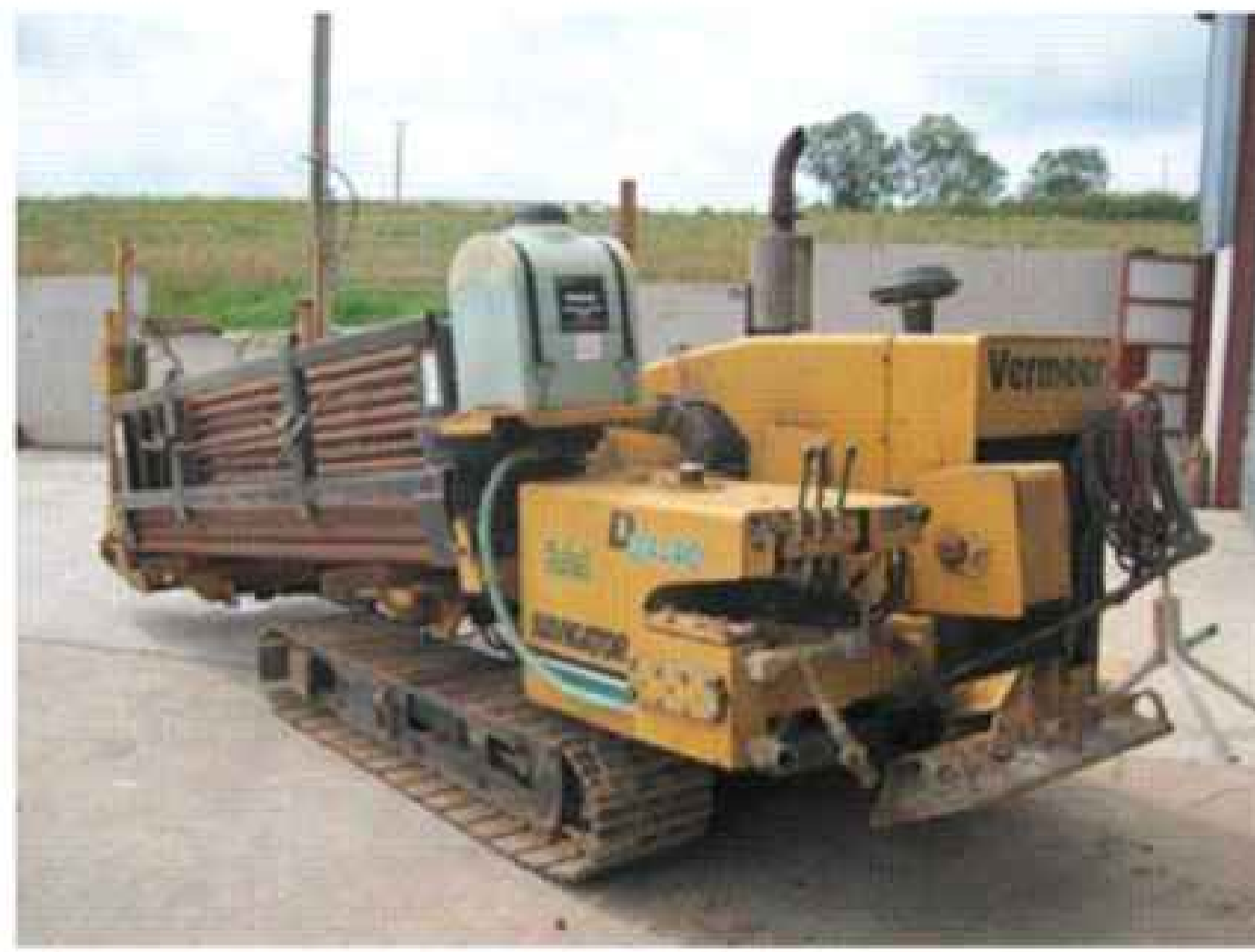
Image 2 | Typical Directional Drilling Rig
